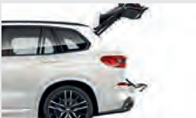
Both the upper and the lower part of the Tailgate can be opened and closed electrically. This facilitates access and loading of the luggage compartment.
