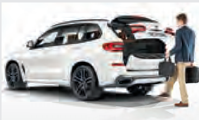
The Comfort Access System makes it possible to open all of the vehicle doors without using the key and to start the vehicle by pressing a button, while the key remains in the pocket. The tailgate can be opened and closed without even being touched with a quick wave of the foot under the rear bumper.
