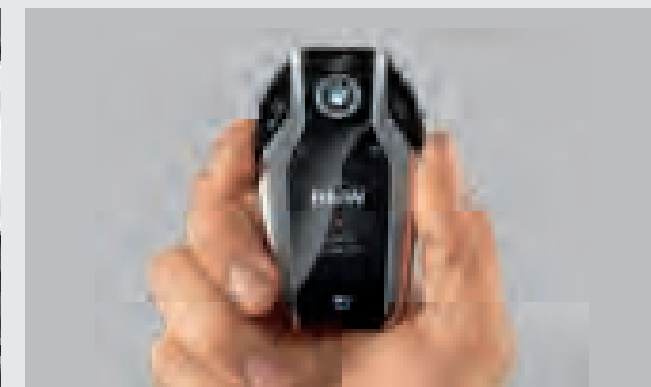
The BMW Display Key shows various information about the vehicle's status and allows selected functions to be controlled with an integrated touch display.
