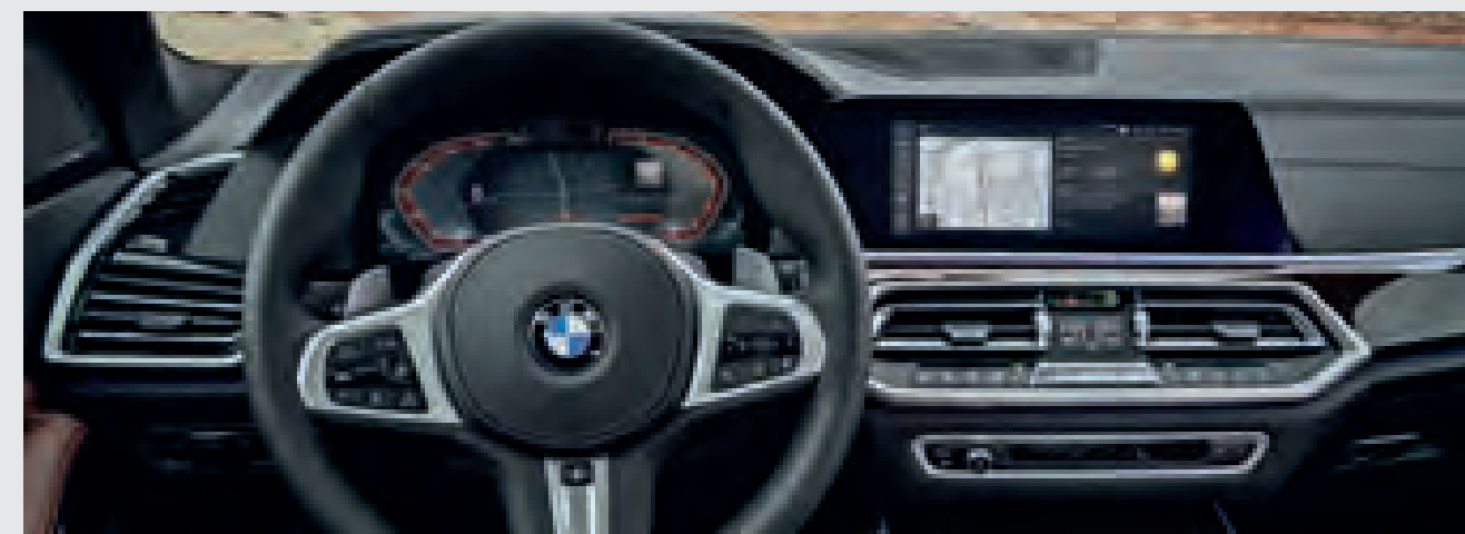
The BMW Live Cockpit Professional with navigation function includes a high-quality display network consisting of a high-resolution 31.2 cm (12.3 inches) Info Display that can be operated by touch and a fully digital 31.2 cm (12.3 inches) instrument cluster.
