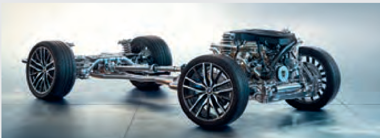
The Adaptive 2-axle Air Suspension ensures extremely comfortable driving with great driving dynamics. The air suspension automatically keeps the vehicle at a constant height, regardless of the load. The driver can raise or lower the vehicle in an adjustment range of approx. 80 mm via a toggle switch in the centre console or via BMW Display Key.
