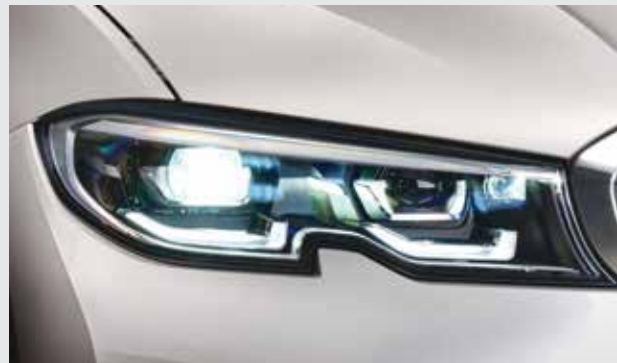
The Adaptive LED Headlights with cornering lights generate a bright and efficient bi-LED light for low and high-beam headlights. The bend lighting and cornering lights with LED technology allow for adaptive light distribution with increased side illumination for city driving. The LED day time running lights and parking lights in the light tubes of the main headlights create a distinctive feature characteristic of a BMW.
