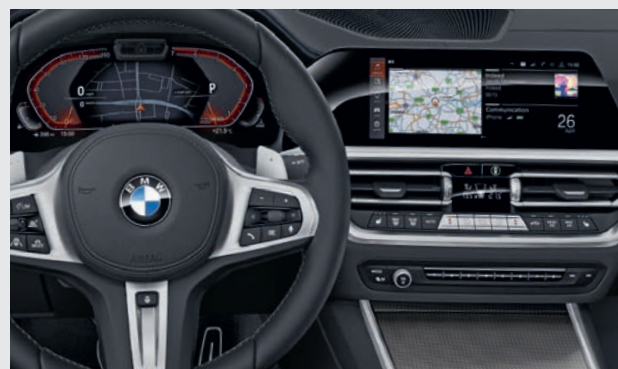
The BMW Live Cockpit Professional with navigation function includes a high-quality display network consisting of a high-resolution 10.25" (26 cm) Control Display that can be operated by touch and a fully digital 12.3" (31.24 cm) Instrument Display. The BMW Operating System 7.0 can also be operated via the iDrive Controller.
