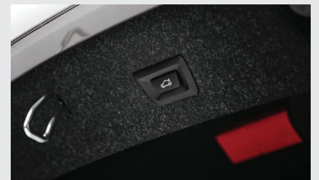
The Automatic Tailgate opens and closes at the press of a button from within the vehicle, as well as with the vehicle key. An additional button for closing the tailgate is located on its exterior.
