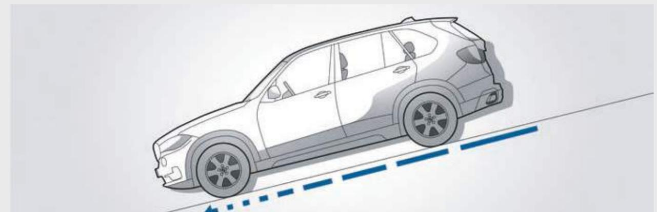
The **Hill Descent Control (HDC)** in the BMW X5 is a system which, when activated ensures that the vehicle can master the steepest downhill runs automatically and safely at just above walking pace, without the driver having to brake.
