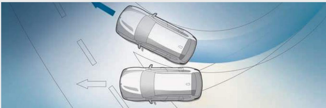
**Dynamic Stability Control (DSC)** permanently assesses the vehicle’s movements and stabilises it using engine and braking regulation when unstable driving conditions are detected. Additional features of DSC are, for example, brake drying, braking readiness or the Hill-Start assistant, which holds the vehicle briefly in place when starting on inclines to prevent it from rolling backwards.
