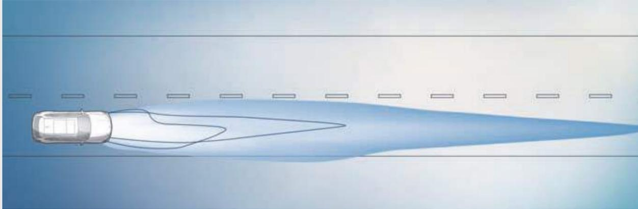
In laser high-beam mode, **BMW Laserlight with X Signature** illuminates a range of up to 600 m, nearly twice as far as that of conventional headlights. Better visibility in the dark significantly increases safety. The blue X signature and the “BMW Laser” lettering underline the vehicle’s technological standards.
